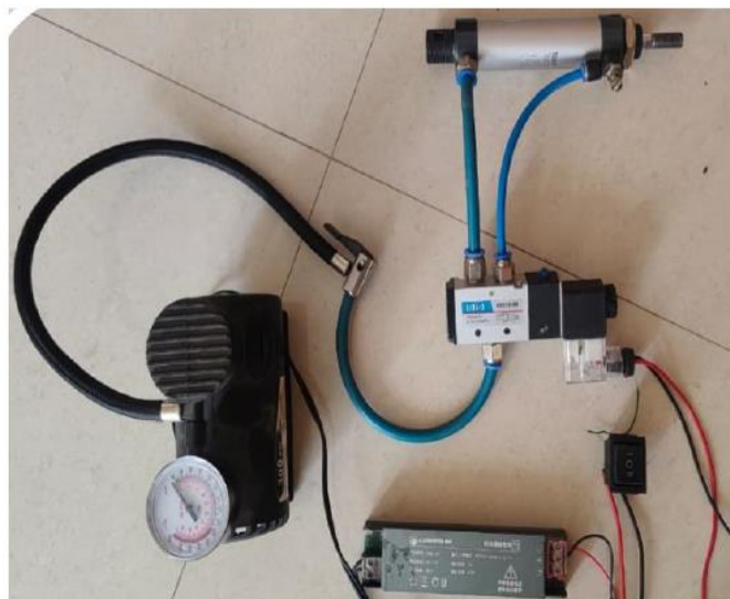
Fig. 3. Experimental Setup of Pneumatic Actuation System.
