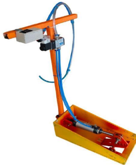
Fig 4: Developed Prototype of Pneumatic Slag Removal System.
