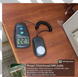
Fig2: Classroom LUX level
